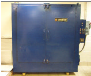
Figure 2: Inner layer baking oven installed in Multilayer lamination room
